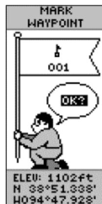
A Waypoint can either be marked to record where you are at that time, or entered into the GPS as somewhere to be heading towards. If you have the required software and connection you can download waypoints from your computer. Without this, they must be entered manually using the GPS controls. Once entered,
